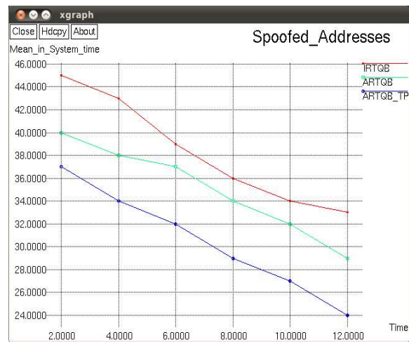
Figure.16. Comparison of Mean in System Time between IRTQB, ARTQB and ARTQB-TP techniques for Spoofed Address Strategy
