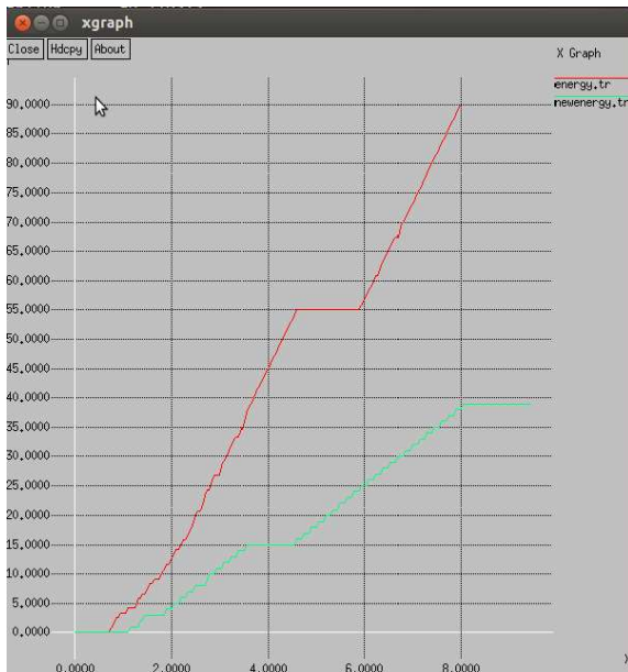
Fig 9: Comparison of energy consumption for AODV and R-optimal algorithm in highway scenario
