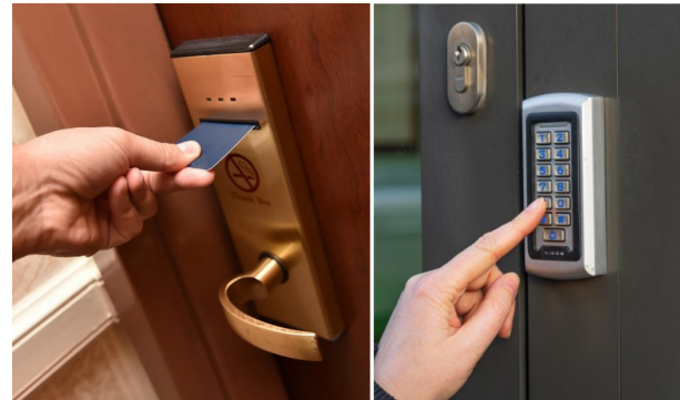
Fig. 3: A door lock where the proof factor is a card [13] (left) and a door keypad where the proof factor is a numeric code [14] (right).
