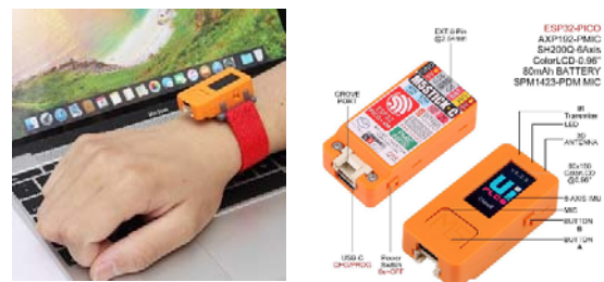
Figure 5 The used M5StickC ESP32 Mini IoT nodes
