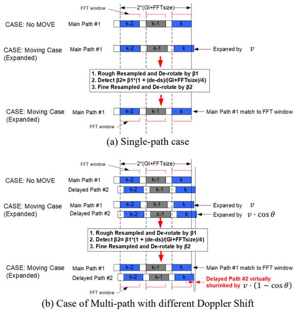
Fig. 4: OFDM signal after the Shrink and Expansion processing
