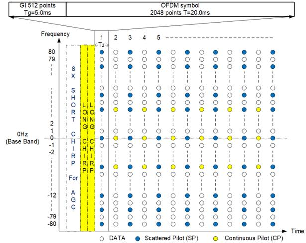
Fig. 2: Time-Frequency structure of OFDM signal
