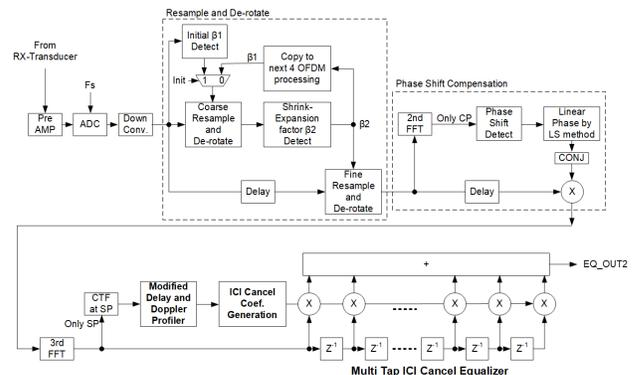
Fig. 3: Receiver Block Diagram with ICI Canceling Equalizer
