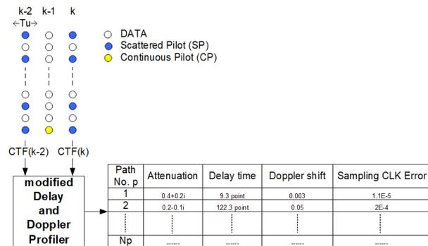
Fig. 5: Modified Delay and Doppler Profiler
